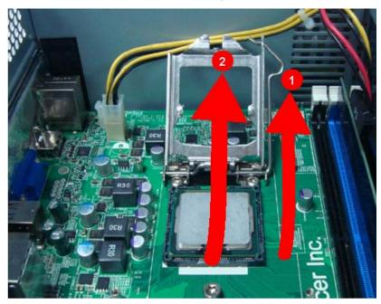
**3.** Pull out the processor from the socket.
